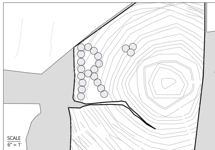
D3 - 22 CAL. SHELL CASING "GRAFFITTI" (NORTH ELEVATION - MID WALL - COURSE # 5)
