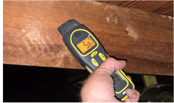
Fig.II.75 Spot checks revealed acceptable moisture content readings throughout the attic.
