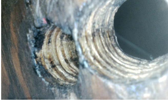
Fig.II.157 The regular ring pattern on the inside of these holes strongly suggests the separate layers of plywood versus actual wood.
